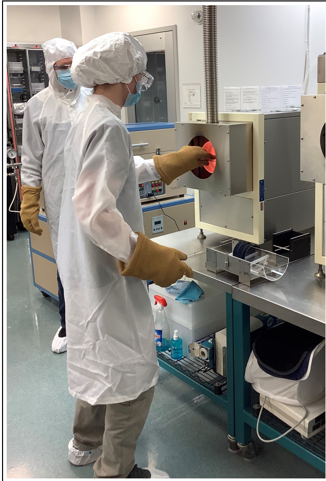
Figure 2. Inserting the Cell into the Furnace
